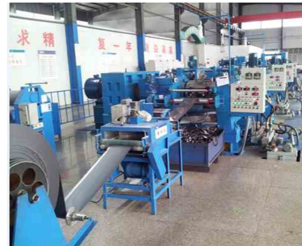
两辊出片机 Two Roll Calender for magnet material sheeting
